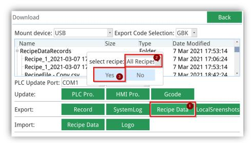
6. When the process is finished, the next message appears, and the csv file is created in the root folder of USB or SD card
