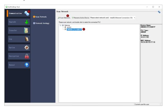
Using this tool it is possible to read or write files in the internal memory of the AM600. These files can then be used in the internal program of the AM600 accessing to this folder /AM600-nand/share/.
